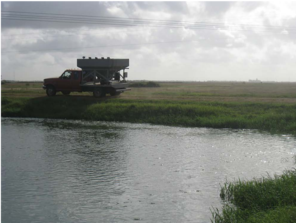
Fig. 8.15. A truck pulling a mechanical feed blower on a pond bank.
