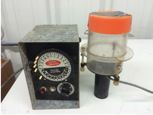
Fig. 8.14. Vibrating feeder with timer. The frequency of feeding can be controlled by the timer and the quantity of feed dispensed is adjusted based on the gap above the vibrating plate and cylinder which contains the feed.
