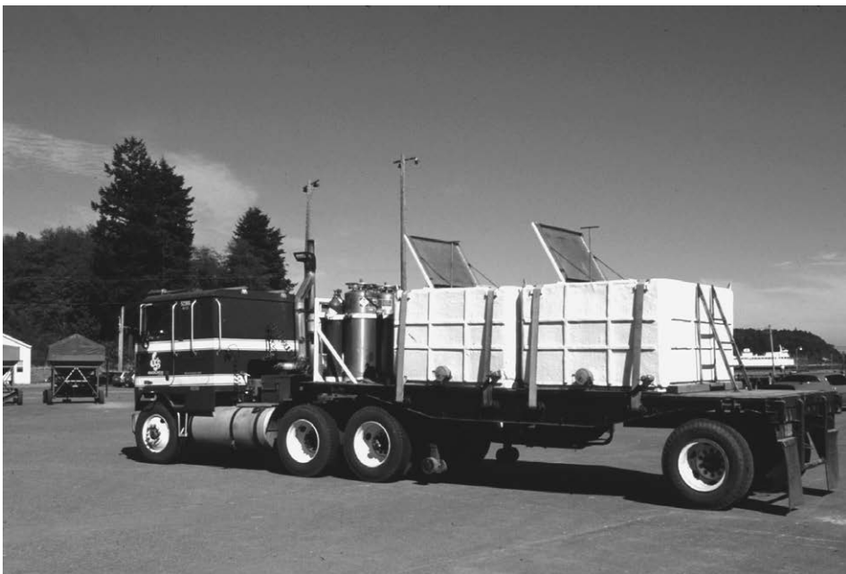
Fig. 9.3. A tractor-trailer unit with insulated hauling tanks.
