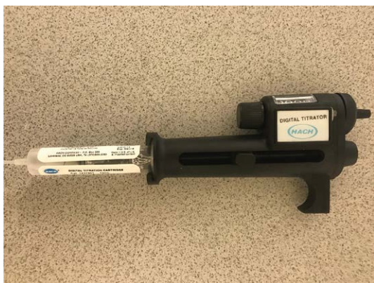
Fig. 4.9. A digital titrator for measuring alkalinity.
