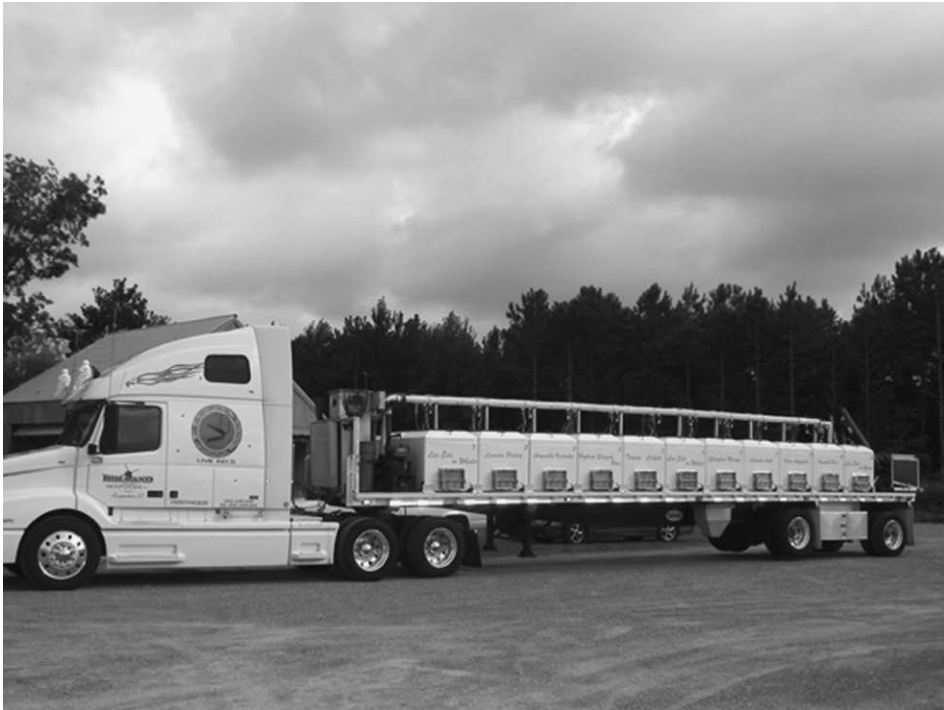
Fig. 9.2. A tractor-trailer unit with tanks that is used to haul live fish.
