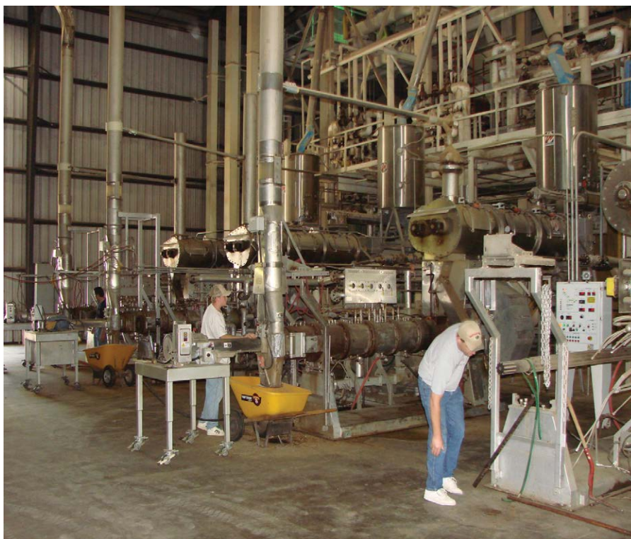
Fig. 8.1. Several extruders operating at a commercial feed mill.
