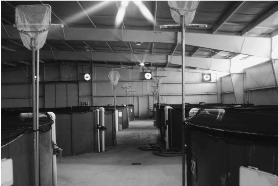
Fig. 5.1. A group of circular tanks in a building, each of which has its own dedicated dip net to avoid cross-contamination.
