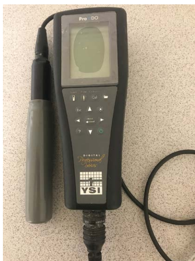
Fig. 4.6. An optical DO meter.
