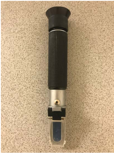
Fig. 4.8. A refractometer for measuring salinity.
