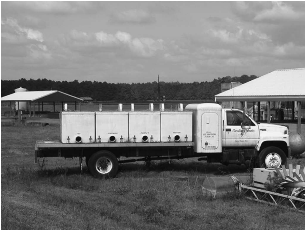
Fig. 9.1. A medium-sized fish-hauling truck.
