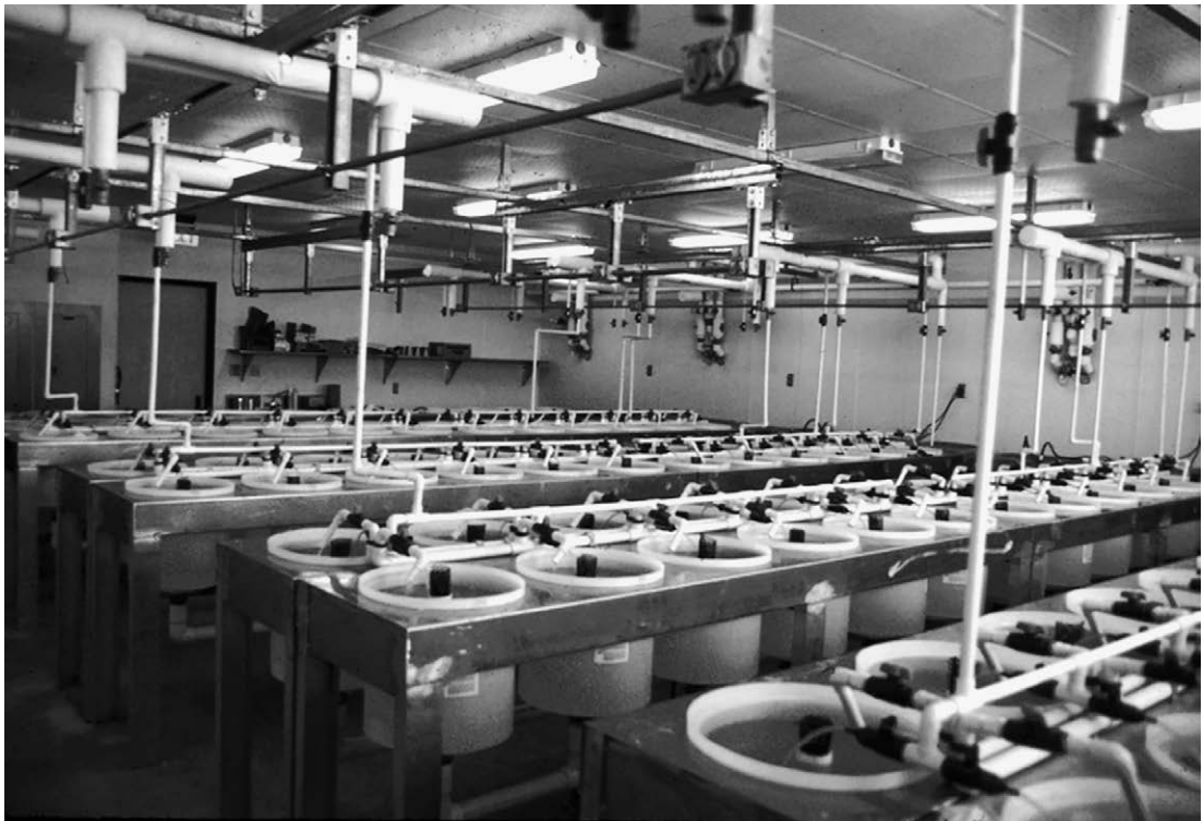
Fig. 3.11. Small circular raceways in a research laboratory.
