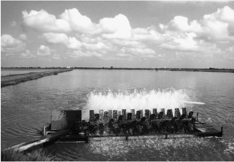
Fig. 4.1. A large paddlewheel aerator at the end of a pond causes the water in the pond to circulate.
