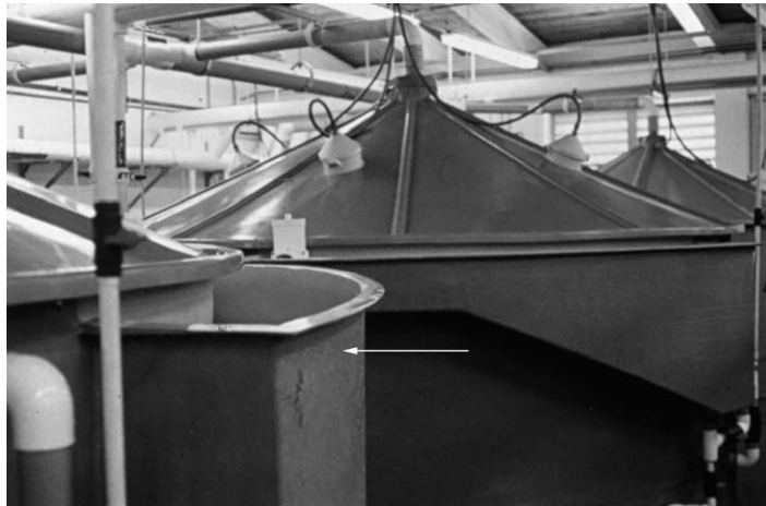
Fig. 6.17. Red drum spawning tanks in a temperature-controlled hatchery room to condition adults to spawn out of season by manipulation of light and temperature (arrow identifies the location of the egg collection box).
