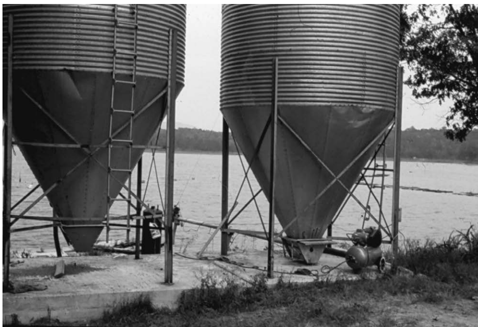
Fig. 5.5. Dry pelleted feed storage bins beside a lake where fish were being commercially produced in cages.
