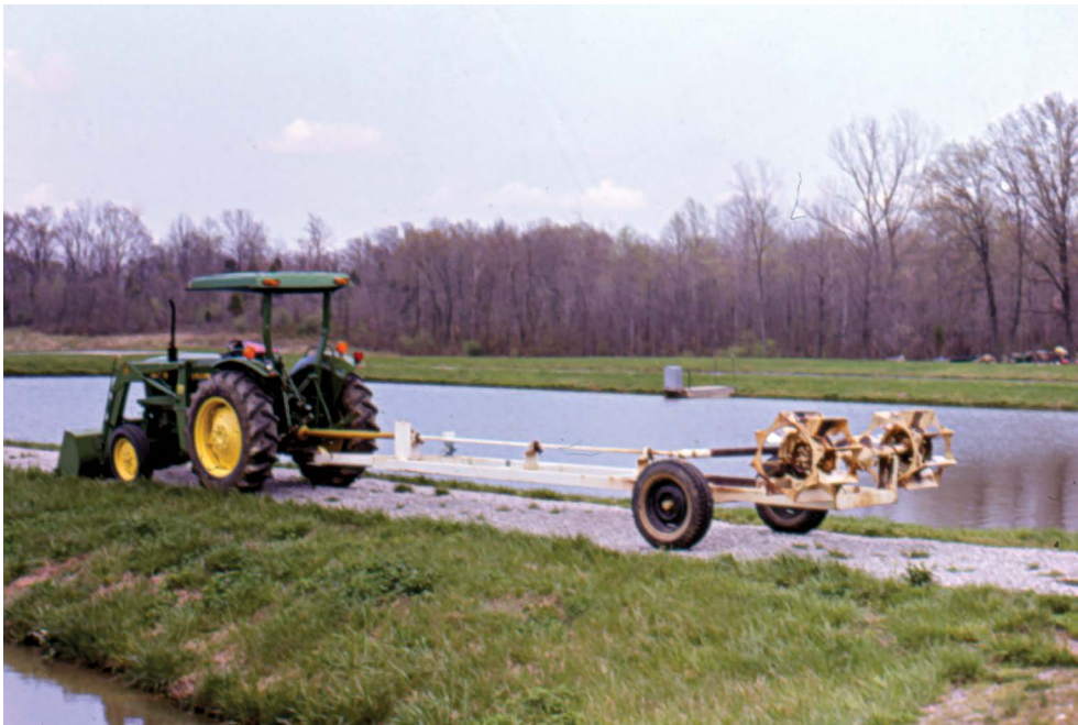
Fig. 4.2. A tractor pulling a paddlewheel aerator.
