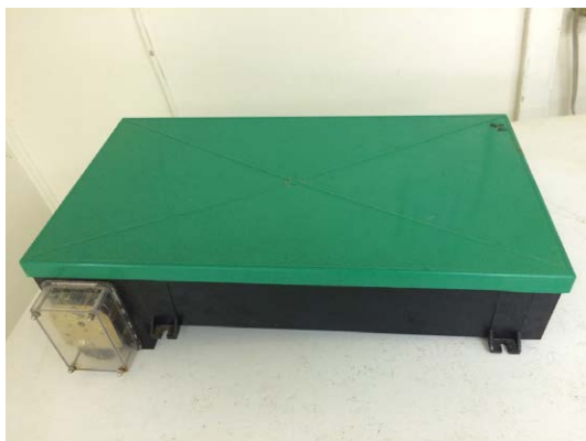
Fig. 8.16. Belt feeder which can be loaded to dispense feed on a continuous basis. Such feeders are available commercially and can also be built relatively easily by the aquaculturist.
