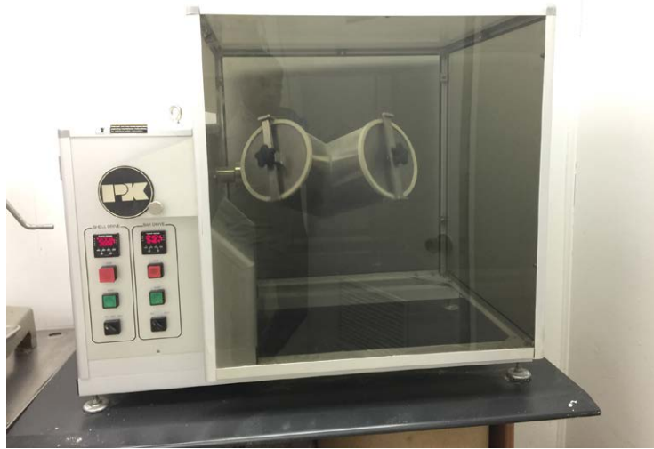
Fig. 8.8. Experimental V-mixer for homogenizing small quantities (up to 3 kg) of dry ingredients.
