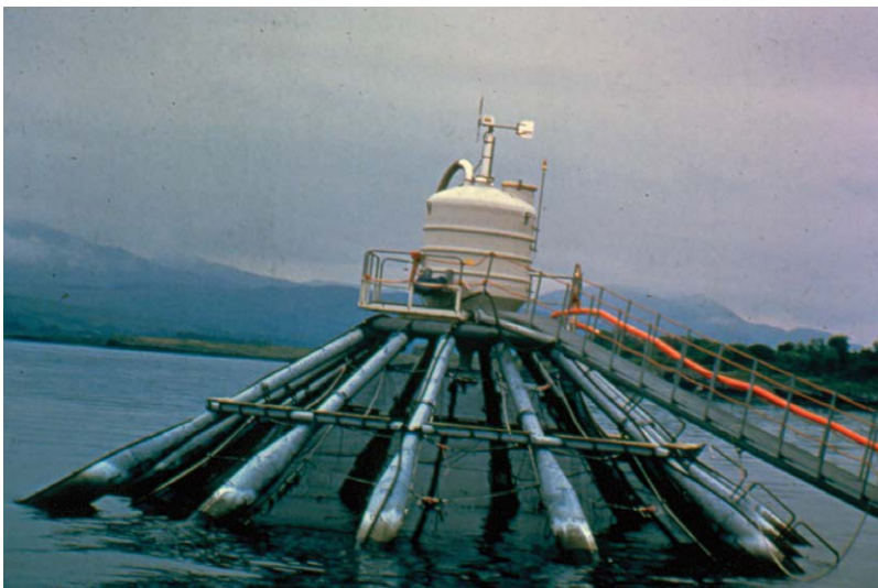
Fig. 3.30. Net pen in Scotland with automated feeding system. The system is designed for operating in the open ocean.
