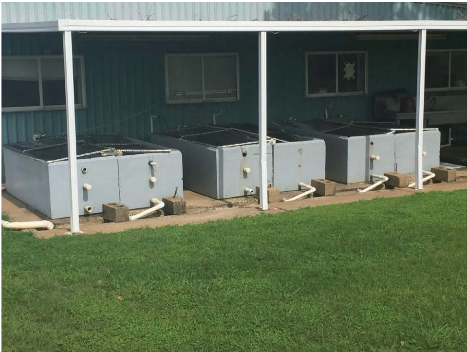
Fig. 3.20. Concrete burial vaults modified for use as experimental tanks.
