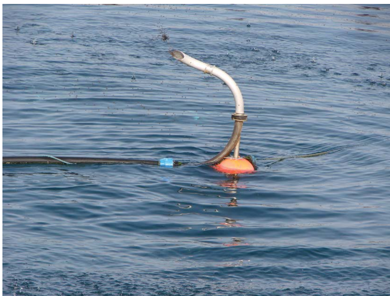
Fig. 8.19. A rotating feed distributor at a net pen.
