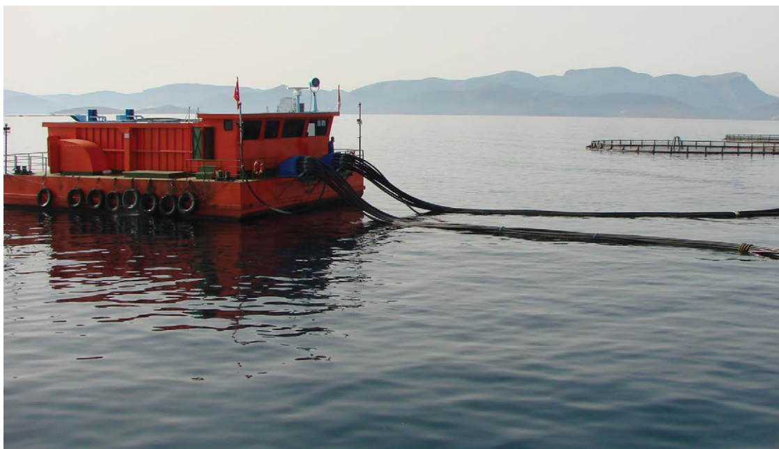
Fig. 8.17. Feed barge with pneumatic tubes for conveying the feed to various net pens.
