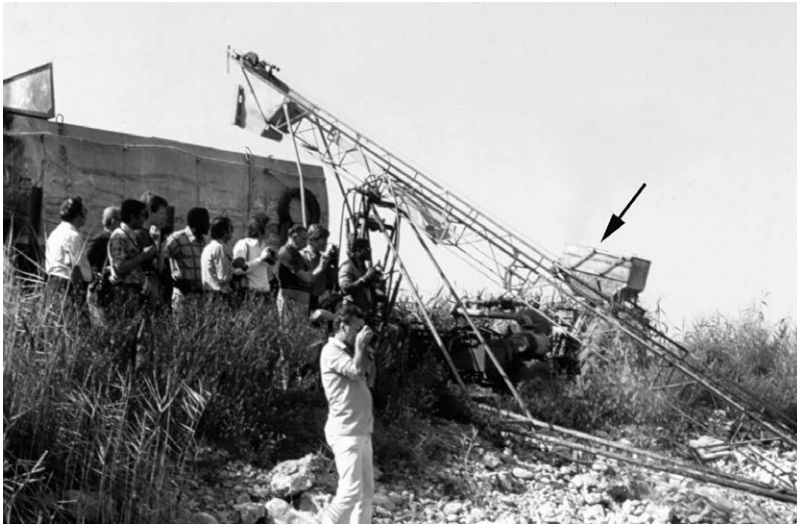
Fig. 9.9. A cart loaded with tilapia (see arrow) moving up the conveyer to be loaded into a live-hauling truck.
