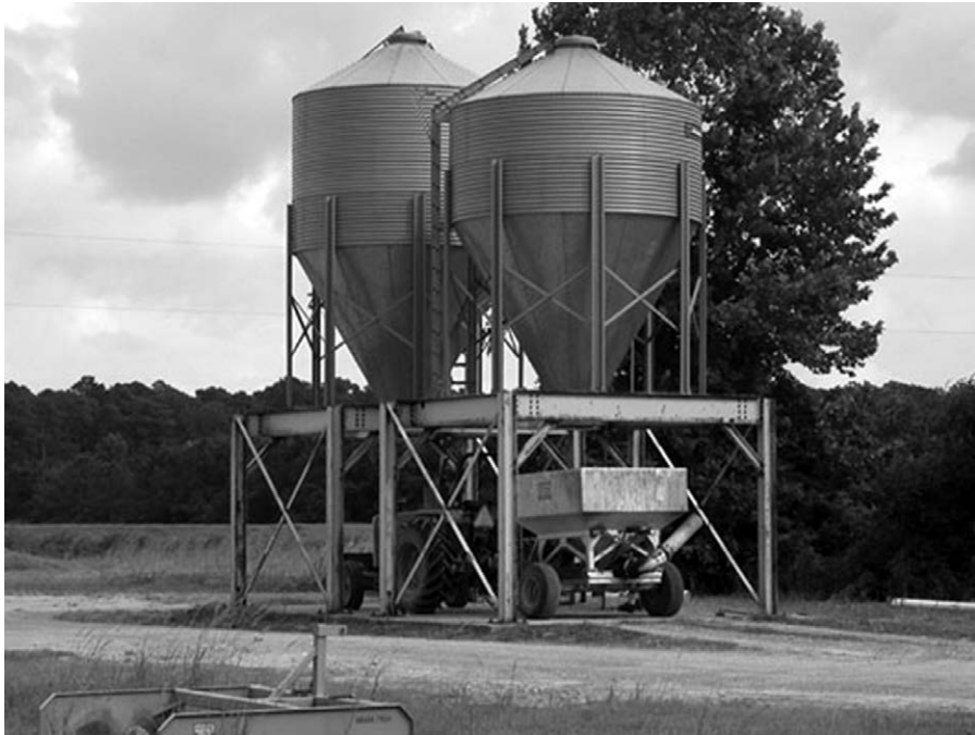
Fig. 3.32. Trailers equipped with feed blowers are often used for feeding large ponds.
