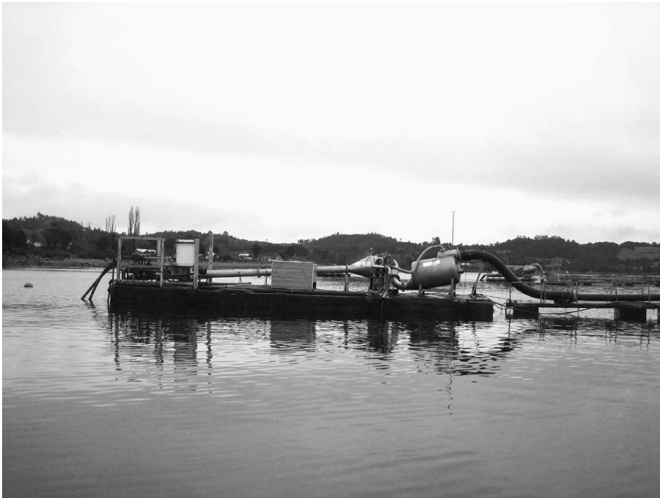
Fig. 9.14. A fish pump at an Atlantic salmon net pen facility in Chile pumps harvested fish from a 'resting' pen into a chilling tank outside the processing plant.
