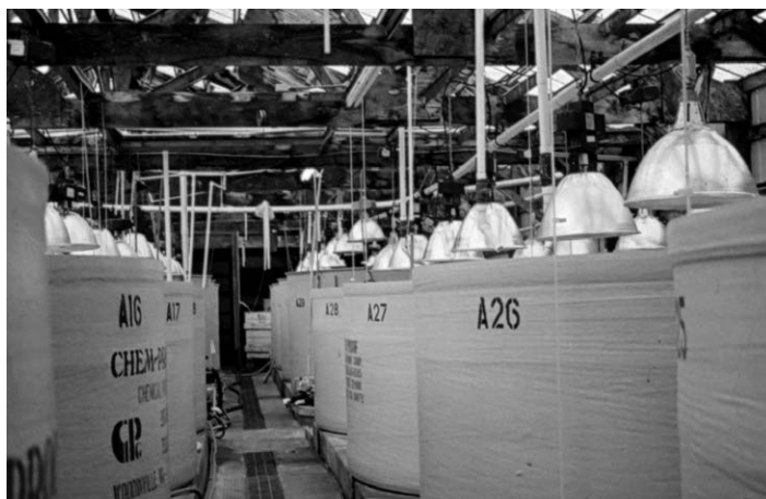
Fig. 6.31. Relatively small batch cultures are used to initiate the large tank cultures of algae that are shown. Note the overhead lights that are required to stimulate photosynthesis. Aeration keeps the algae in motion.
