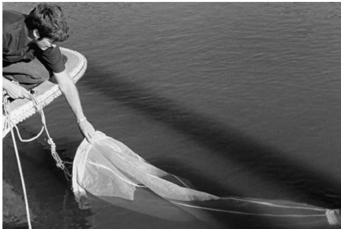
Fig. 6.33. Plankton nets can be used to collect wild zooplankton. The nets are available in various mouth diameters (with 0.5 and 1.0 m being common) and mesh sizes. A cup at the end of the net collects the sample.
